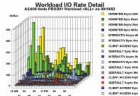
Workload I/O Rate Detail BMC PATROL for iSeries - Perform shows the average I/O per second for each workload
